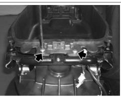
• Undo and remove the screws fixing the helmet compartment - license plate.
