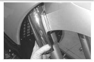
• Unscrew and remove the screw fixing the speed sensor and collect the nut.
