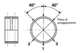
Before fitting, check that the clearance between the engine crankcase bushing and the crankshaft is within the predetermined limits.
