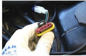
Checking under regular functioning by placing the specific tool between the pump and the injector. With >12V battery voltage, check that the fuel pressure is 3 BAR and that the input current is ~2.8 A
