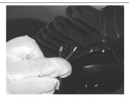
• Remove the helmet compartment light bulb.
