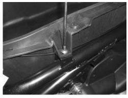
• Undo and remove the two rear screws.
