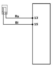
With the wiring disconnected from the control unit and connected to the system, check that the sensor resistance between pins 13 - 15 is between 100 and 150 Ohm at an engine temperature of about 20°
