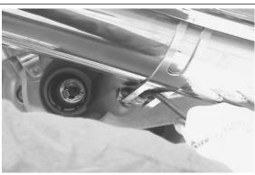
• Undo and remove the exhaust end fixing screw.
