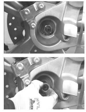
• Unscrew and remove the two front nuts fixing the muffler supporting plate.
