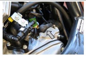
• Disconnect the coolant temperature sensor.
