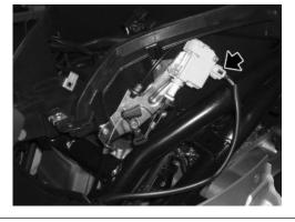
• Disconnect the saddle opening - actuator control cable.
