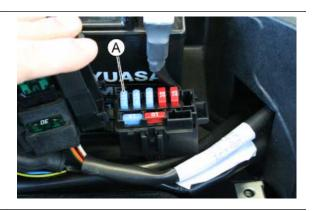
Check the efficiency of the injection load remote control: Check the resistance of the drive coil between pins 86 and 85: 40 ÷ 80 Ohm. Apply a voltage of 12V to pins 86 and 85; make sure that there is continuity between pins 30 and 87 of the remote control.
