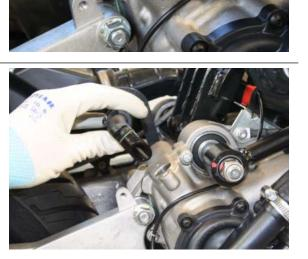
• Undo the screw of the air filter internal support.
