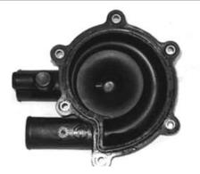
• Place a new O-ring with caution so that it does not come into contact with any grease or oil.
