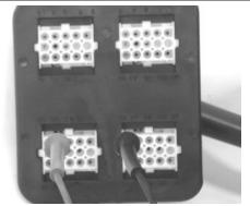
Check the resistance of the coil primary between pin 22 of the interface wiring and the Red-Brown cable of the injection load remote control base, with both the control unit and the remote control disconnected.
