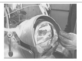
• Undo and remove both screws fixing the headlamp to the chassis.
