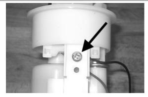
Remove the clip fixing the piping to the filter shown in the photograph
