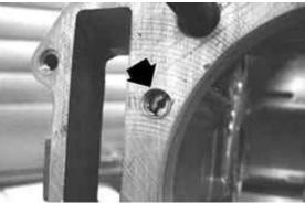
Jet clogging impairs head lubrication and the timing mechanisms.
