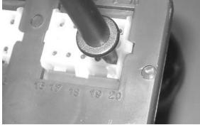
Check there is voltage between the Green-Red cable of the remote control base and the ground lead.
