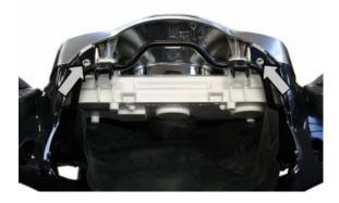
• Remove the front handlebar cover.
