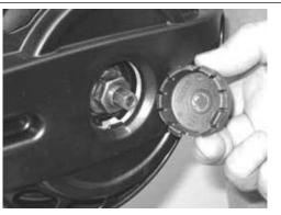
NOTE CHECK THAT THE AIR INTAKE AND OUTLETS ARE COMPLETELY FREE. - Fit the plastic external transmission cover.
