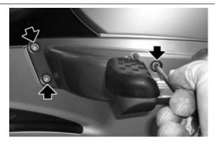
• Remove the screw «1» placed under each footrest.
