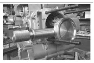
NOTE THE TOOL FOR INSTALLING THE STOP RINGS MUST BE USED MANUALLY. CAUTION USING A HAMMER MAY DAMAGE THE RINGS HOUSINGS.
