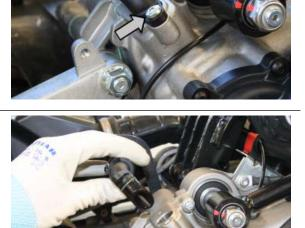
• Undo the air filter internal support screw.
