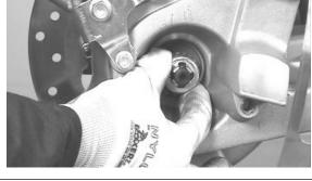
With the help of a second operator, operate the rear brake; unscrew and remove the rear nut fixing the muffler supporting bracket.
