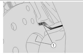
• Replace both pads if the friction material thickness (even in only one pad) is reduced to about 1.5 mm.
