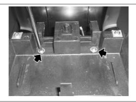
• Working on both sides, undo and remove the side screws.
