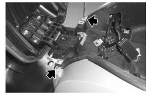
• Working on both sides, undo and remove the two side lower fixing screws.
