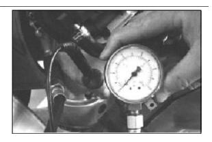
5 - Measure pressure with cold and idling engine.
