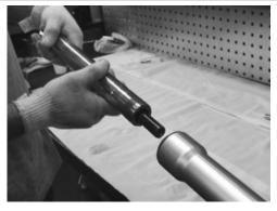
Slide off the pumping member «2» from the stem and collect the spring «3».
