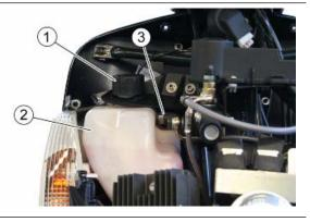
Make sure that the coolant level in the expansion tank «2» is between the «MIN» and «MAX» reference marks.
