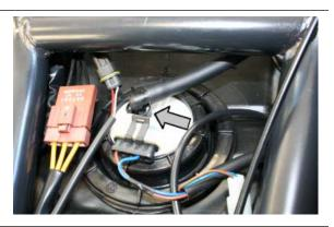
• Working on the left side, disconnect the electric connector and working on the right side, slide off the pipe.
