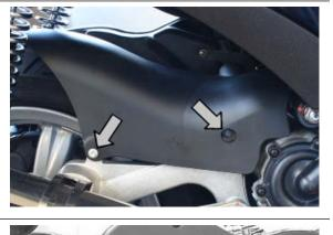
Undo and remove the screw fixing the oil scavenge flange.
