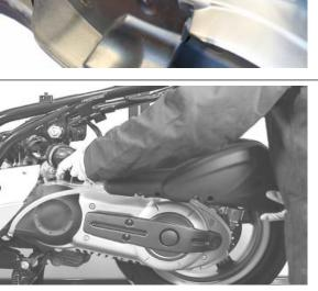
Detach the shock absorber. • • Undo the lower screw fixing the rear left shock absorber and collect the nut. Detach the shock absorber. • • Loosen the set screws and slide off the throttle control cables.
