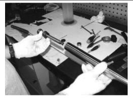
• Insert the stem together with the bushing «2» in the sleeve.
