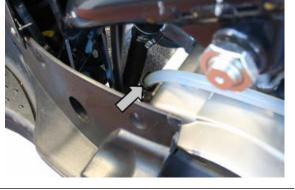
• Remove the filter housing.
