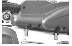
• Undo and remove the oil scavenge flange fixing screw.
