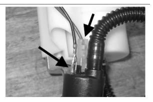
Remove the screw indicated in the photograph
