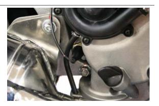
Working on both sides, undo and remove the side screw fixing the chassis central cover.
