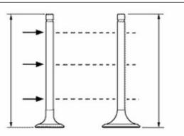
Check the deviation of the valve stem by resting it on a « V »-shaped support and measuring the extent of the deformation using a dial gauge.
