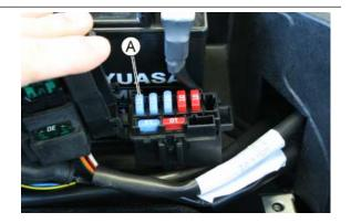
Check the efficiency of the injection load remote control: Check the resistance of the drive coil between pins 86 and 85:  $40 \div 80$  Ohm. Apply a voltage of 12V to pins 86 and 85; make sure that there is continuity between pins 30 and 87 of the remote control.
