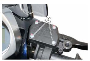
Remove the pump cover with its gasket and top-up the reservoir only with recommended fluid.
