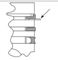
Oil scraper ring: Standard coupling clearance: 0.01÷0.06 mm Maximum clearances allowed after use: 0.10 mm If clearances measured exceed the maximum values specified in the table, the piston should be
