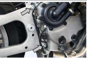
• Remove the muffler supporting plate.
