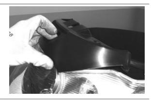
• Undo and remove the two rear screws fixing the tail section.
