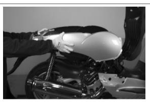
Once the tail section is removed, the fairings can also be removed by loosening the three screws indicated on both sides.
