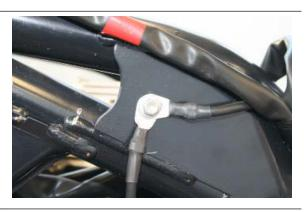
Upon switching to "ON", check that there is battery voltage for about two seconds between the Red-Brown cable of the pump connector and ground connection, with the pump connector disconnected. Otherwise, check the continuity of the Red-Brown cable between the pump connector and the remote control base.
