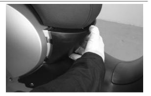
• Undo and remove the two front screws fixing the tail section.
