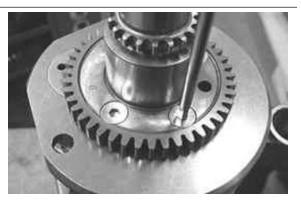
Blow with compressed air and degrease the mounting holes on both surfaces to facilitate adherence of the new LOCTITE applied.
