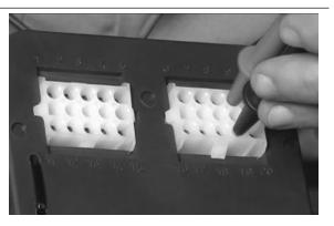
With the control unit-side connector disconnected and the coolant temperature sensor connector also disconnected, check the continuity between pin 9 of the interface wiring and the Orange cable of the connector.
