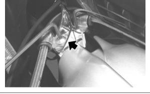
• Undo and remove the internal screw of the stem protection.
