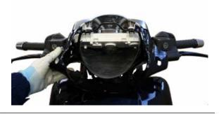
• Disconnect the instrument panel connector.
