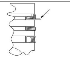
Maximum clearances allowed after use: 0.10 mm If clearances measured exceed the maximum val-
