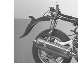
• Undo and remove the upper screw fixing the right shock absorber and collect the nut.
