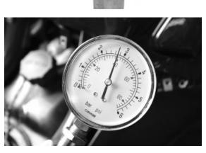
Carry out the injector sealing test Dry the injector outlet with a blast of compressed air. Activate the fuel pump. Wait for one minute and make sure there are no leaks coming from the injector. Slight oozing is normal. Limit value = 1 drop per minute
