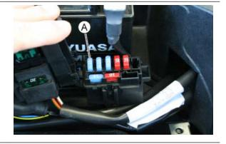
Check the efficiency of the injection load remote control: Check the resistance of the drive coil between pins 86 and 85: 40 ÷ 80 Ohm. Apply a voltage of 12V to pins 86 and 85; make sure that there is continuity between pins 30 and 87 of the remote control.
