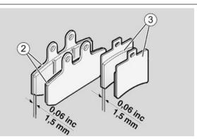
In case of uneven wear, replace the pads when there is a thickness difference of 0.5 mm in the friction material.
