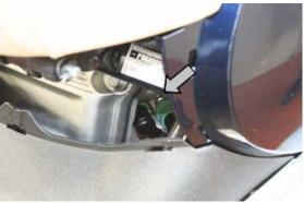
• Remove the injector control sensor.
