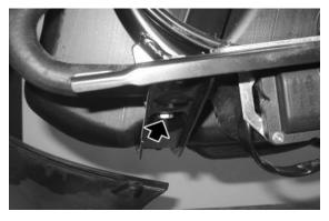
• Undo and remove the front screw fixing the fuel tank.
