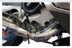
If coolant or oil leaks are detected, inspect the pump (see the «Engine/Water pump» chapter).
