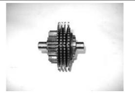
The limiter assembly cannot be overhauled. In case of clearly visible irregularities on the toothed discs, replace the assembly.
