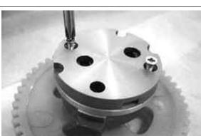
Failure to observe the tightening torque may alter the coupling clearance between the rotors and the pump body.
