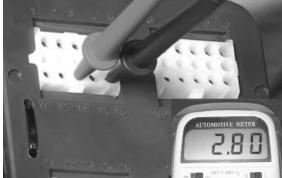
With the interface wiring disconnected from the control unit, check continuity between pin 13 and the Red cable of the rpm sensor connector and between pin 15 and the White cable of the rpm sensor connector.
