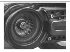
Remove the cap to inspect the TDC reference found between the flywheel and cover housing.
