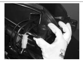
• Slide off the cables from the helmet compartment.
