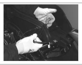
• Undo and remove the fixing screw of the helmet compartment light switch.
