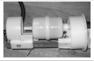
Remove the filter from the pump support
