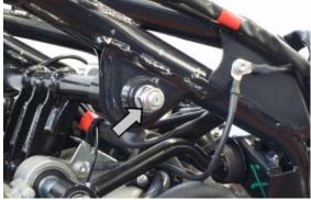
Unscrew and remove the link rod fixing nut and collect the washer and the silent block.
