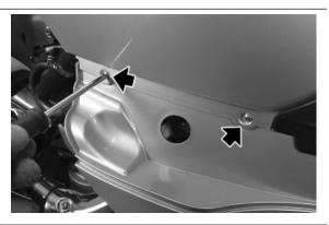
• Undo and remove the four screws fixing the passenger grab handle.
