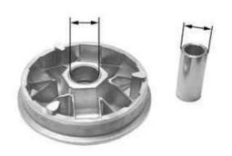
Characteristic Minimum diameter allowed: Ø 29.95 mm Standard diameter: Ø 29.959 mm - Check that the rollers are not damaged or worn. Characteristic Minimum diameter allowed: Ø 24.5 mm Standard diameter: Ø 24.9 mm - Check the guide shoes for the variator roller contrast plate are not worn.
