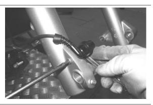
• Loosen the two screws fixing the fork stem.
