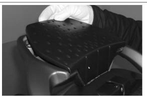
• Undo and remove the three screws fixing the passenger grab handle.
