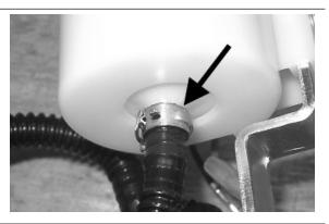
Separate the lower part of the pump support as shown in the photograph.
