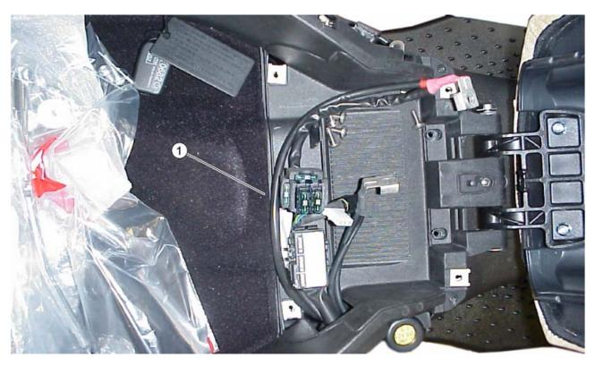
1. Cable harness installation inside the Battery Compartment
