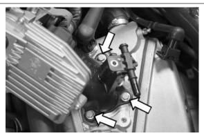
Fit the appropriate tool to check fuel pressure and position the manifold over a graded container, with a minimum capacity of 100 cm<sup>3</sup>. Connect the injector with the cable that is part of the components supplied for the injection tester. Connect the cable terminals to an auxiliary battery. Activate the fuel pump with the active diagnosis. Check that, within 15 seconds, approx. 70 cm<sup>3</sup> of fuel is delivered at a regulation pressure of about 3 BAR.
