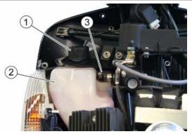
Top-up with coolant until the fluid level is near the «MAX» reference mark.
