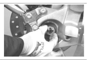
With the help of a second operator, operate the rear brake; unscrew and remove the rear nut fixing the muffler supporting bracket.
