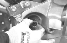
• Unscrew and remove the two front nuts fixing the muffler supporting plate.
